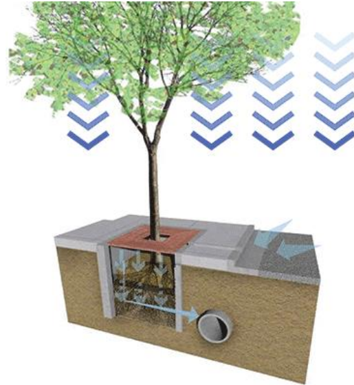
Figure 31. Diagram of a Bioretention adapted from the Houston-Galveston Area Council.
